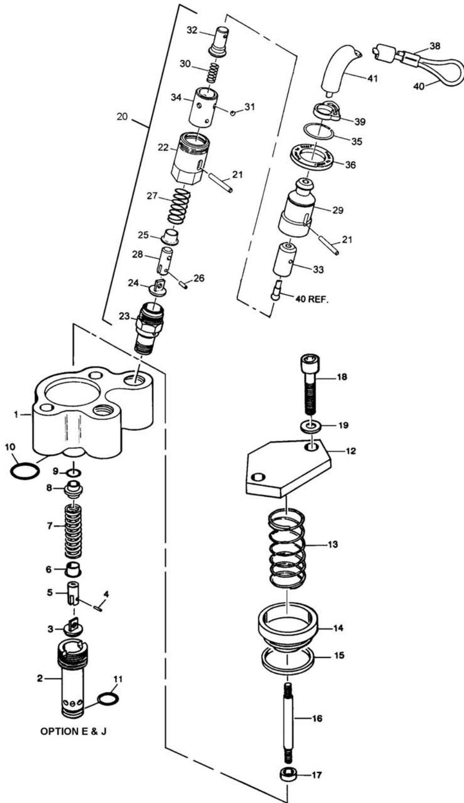
FIGURE 7 - AIR/LANYARD OPERATED PILOT VALVE, OPTION F
