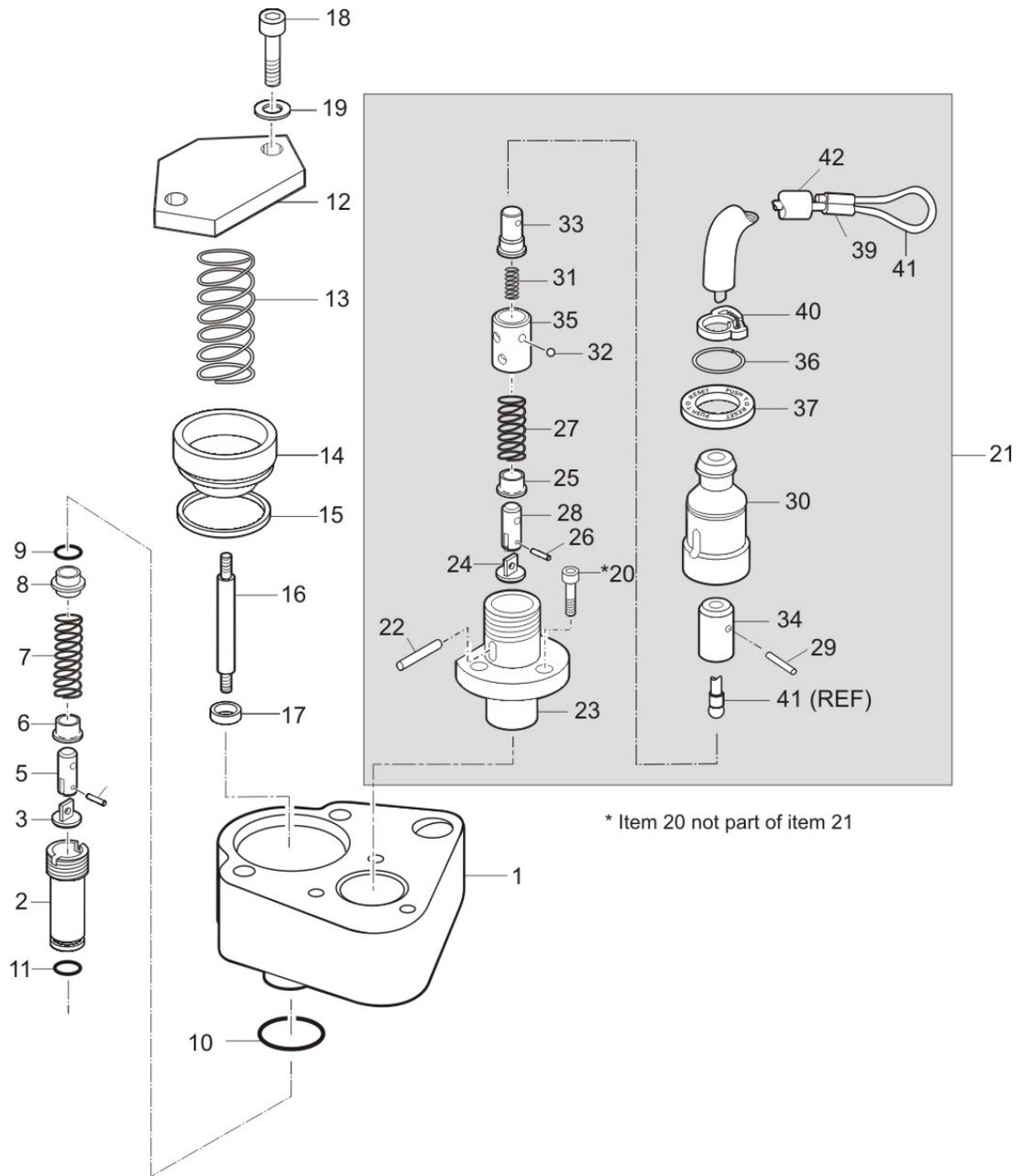
FIGURE 8 - AIR/LANYARD OPERATED PILOT VALVE, OPTION U
